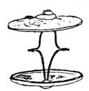
Cut one pair of bell wire 4" long and trim off 1/2" of insulation from all ends. Attach one wire to each pair of connected bulb wires (solder if desired), and wrap the connections with tape.
